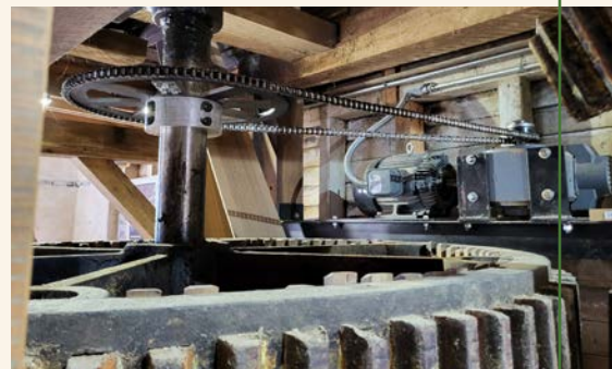
Top to bottom: Jason Pastor (left) and Ari Bortman used computer-aided design in their planning; Pastor and Bortman on the great gear; sprocket and chain above the great gear.
